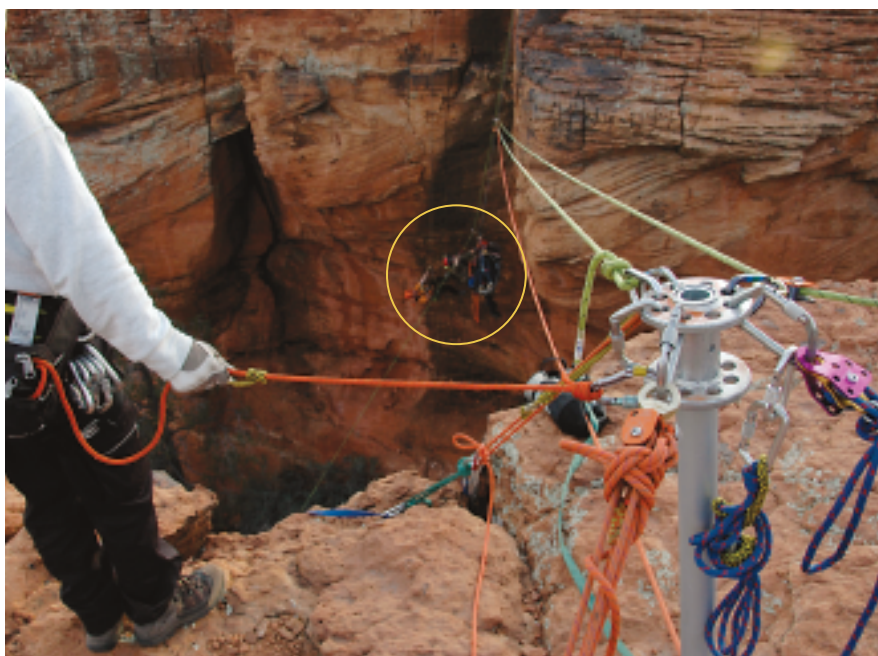
Here, both ends of the AZTEK are used at the same time. 1) A small rigging pod with a compression member to elevate it above the edge beyond is being guyed with two separate AZTEKs. Note how the SOF is always tied off with a mule hitch before the operation. 2) The personal end of the AZTEK is used by a firefighter working near the edge. Note the Purcell travel restrict and double-zipper bag.
