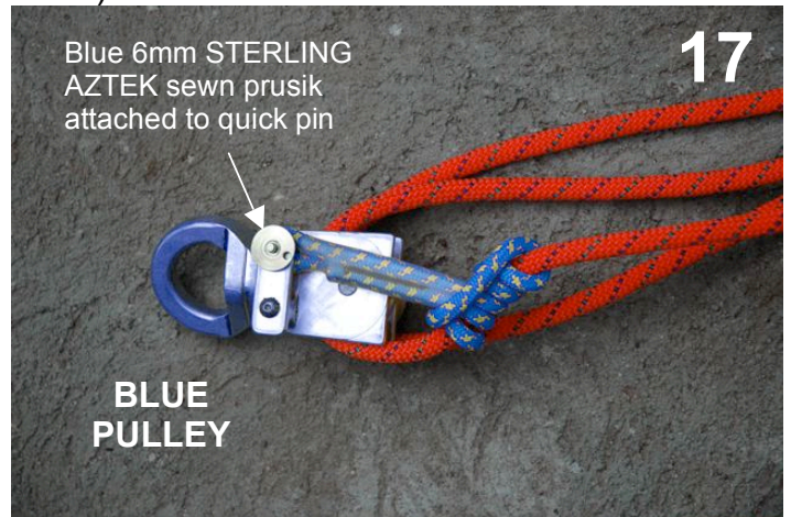
17. Decide which end of set-of-fours to attach ratchet and then remove small quick pin which comes with AZTEK Elite® pulleys
