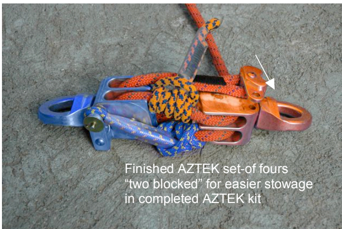
The Rock Exotica Omni AZTEK Elite® SYSTEM END completely collapsed with the customary lineman "reverse reeve". Notice the prusik not used (in this case the orange) floats on the rope during use and cannot be taken from the rope by accident
