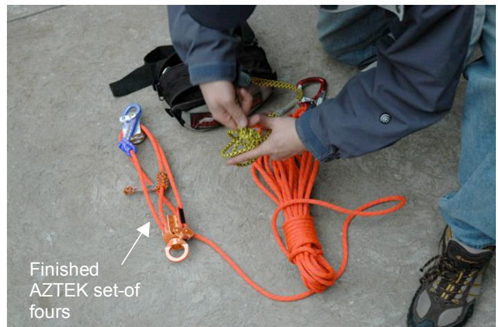
14. Pin in place orange ratchet to orange pulley or blue ratchet to blue pulley. DO NOT attached orange ratchet to blue pulley or vice versa. Only one ratchet should be attached at a time for proper operation.
