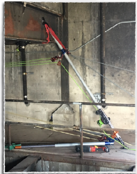
Top right: A rigging jamb pole tripod with SkyHook® capstan winch on one leg using the AZ Vortex (AZV)
