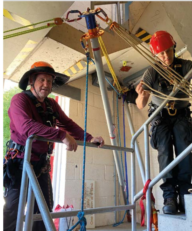
BELOW: Delta guyed gin pole using three AZTEK at 120° angles. Photo from Llangollen, Wales, AHDW workshop with R3 Safety & Rescue in 2022.
